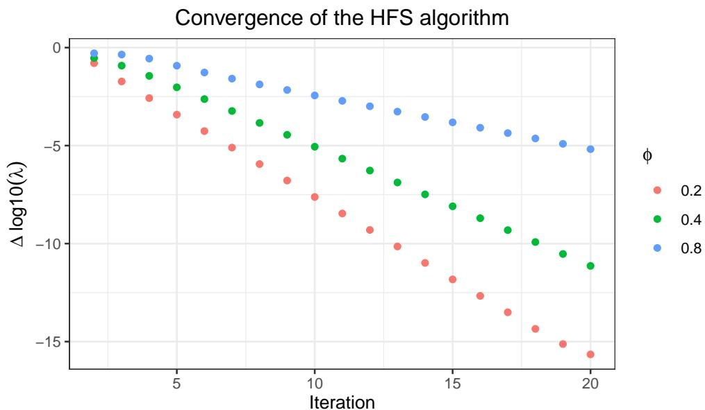
Speed of convergence of the HFS (Harville-Fellner-Schall) algorithm for different values of the standard deviation of the noise ( $\phi$ ) in the simulation. R code in f-HFS-convergence.R
