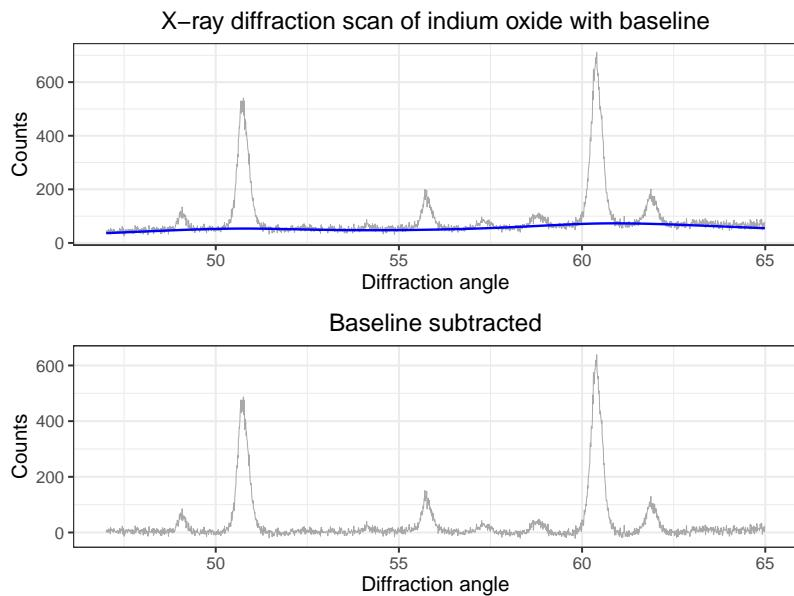
X-ray diffractometry scan of indium oxide. Estimation of a baseline by expectile smoothing with 40 cubic B-spline segments,  $\lambda = 1000$ , and asymmetry  $\tau = 0.04$ . Top: data and baseline; bottom: after subtraction of the baseline. R code in f-baseline.R
