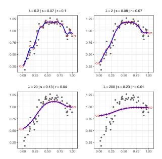
The first order penalty in action for various values of  $\lambda$ . Also shown are the standard deviations of the residuals (s) and the roughness measure (r). Cubic B-splines, 20 segments. R code in f-d1pen.R
