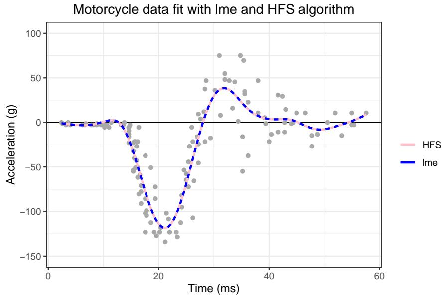
Automatic smoothing of the motorcycle data with a mixed model using the `lme` function (solid blue line) and with the HFS algorithm (broken red line), both with  $\lambda \approx 0.01$ . R code in `f-mot-lme-mix.R`
