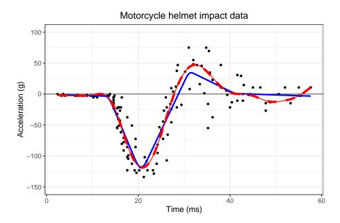
Median smoothing of the motorcycle data using cubic P-splines, with 50 segments on the domain from 0 to 60 ms. The piecewise-linear curve (solid blue line) is obtained with absolute values in the penalty ( $\lambda=10$ ). The smoother curve (broken red line) is obtained with squares in the penalty ( $\lambda=1$ ). R code in f-mot-median-iter.R
