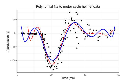
The acceleration of a motorcycle helmet in a simulated crash. Two polynomial (degree 9) fits are displayed. Blue line: based on all data; red broken line: after discarding the observations at less than 5 ms. R code in f-motpol1.R
